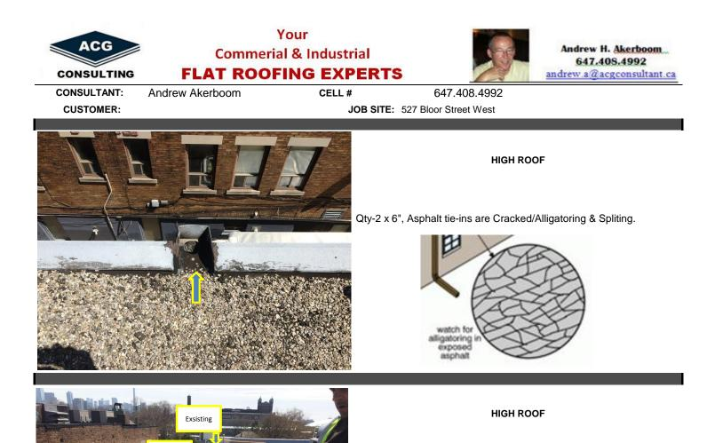
Recommend installing one additional scupper where noted on picture.
